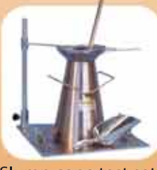
Slump cone test set
