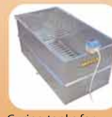
Curing tanks for concrete specimens
